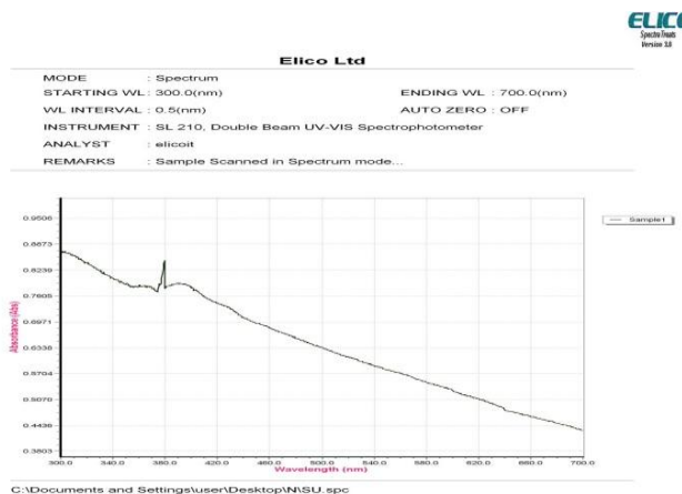
Fig.2. UV-Vis absorption spectra of silver nanoparticles synthesized by Lobophora variegata exposure with 1mM Silver nitrate.
