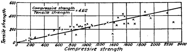
FIG. 1.—Compressive strength vs. tensile strength.
