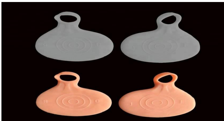
Figure 3:- skin model of silicone used to simulate a human skin in laboratory
