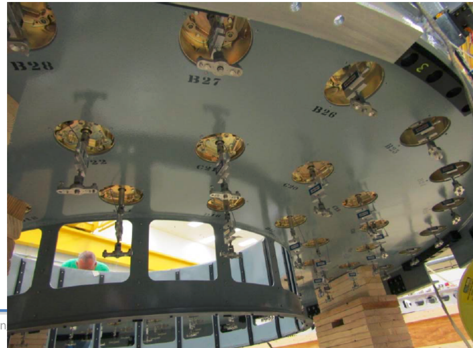
M2 Mirror Cell view from below showing actuator attachments to mirror pads
