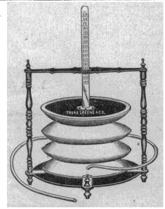
This illustration shows the simplicity of construction. The manometer, which is here attached, should After the large experience I have had with dysen- be used separately. A spirometer gives the vital capacity, viz., the full number of cubic inches possible to be expelled from the lungs after a forced inspiration, while the manometer records the elastic tension which the air cells will stand under a forced expulsion of air from the chest, as compared with the average of a healthy man.
