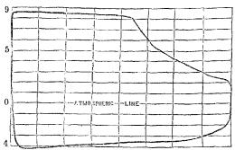
It will be observed, that the double strokes of piston were nearly in the proportion of the square roots of the effective pressure on it.
