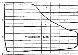
No. 3. Initial steam pressure in cylinder per square inch of piston above atmosphere,  $25\frac{1}{2}$  pounds; cut off at  $^{9}_{16}$ ths stroke of piston. Mean effective pressure throughout stroke of piston,  $30\frac{1}{2}$  pounds. Double strokes of piston, 20 per minute.
