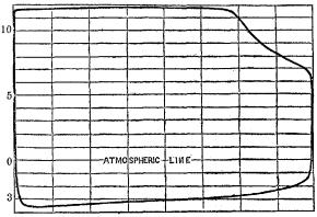
No. 2. Initial steam pressure in cylinder per square inch of piston above atmosphere, 29 pounds; cut off at full three-eighths stroke of piston. Mean effective pressure throughout stroke of piston,  $30\frac{1}{2}$  pounds. Double strokes of piston, 20 per minute.
