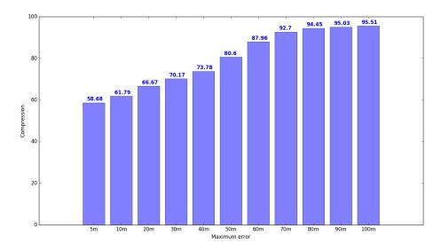
Fig. 2. Data compression as a function of the maximum distance error when when compared to the complete raw AIS positional dataset
