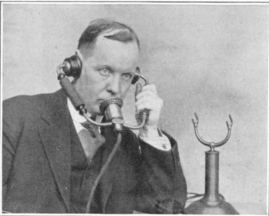
How the anti-noise transmitter is applied to regular telephony. The receiver mechanism, in this case, is located in the base of the hand set
