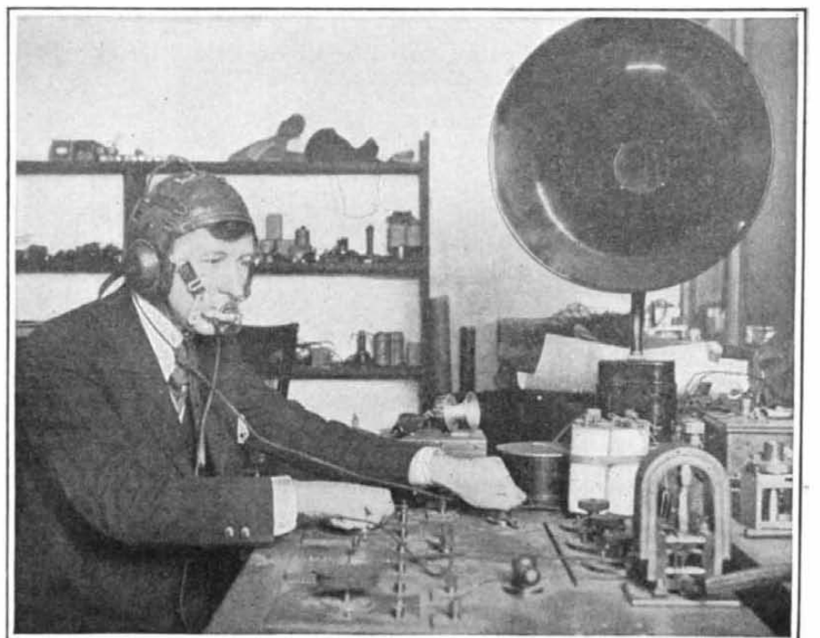
How the aviator wears the anti-noise transmitter, and the special loud-speaking telephone which operates on a new principle
