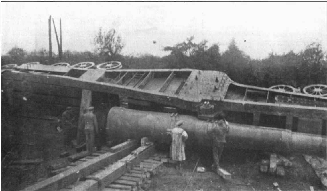
DERAILMENT OF 12IN. GUN (ON RAILWAY MOUNTING). FIG. 9.
