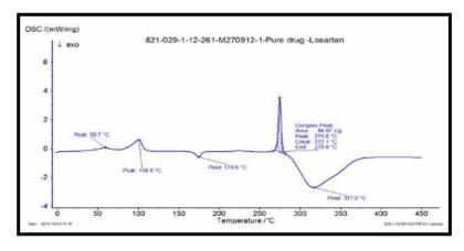
$Fig.\ 7: DSC\ Thermogram\ of\ Losartan\ Potassium.$
