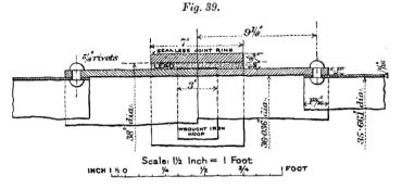
admitted of curves of comparatively small radius being followed in laying such a main, without specials. The difficulty anticipated from the flowing of the lead through the joints of the pipes was entirely overcome by the insertion of a temporary band of iron
