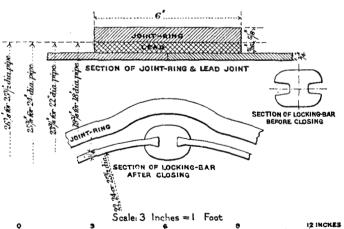
expanded in the pipe by means of a screw, and such a joint was certainly not more expensive to caulk than that adopted on the Coolgardie works, while the use of spun yarn-a perishable material-was entirely avoided. With regard to the method of
