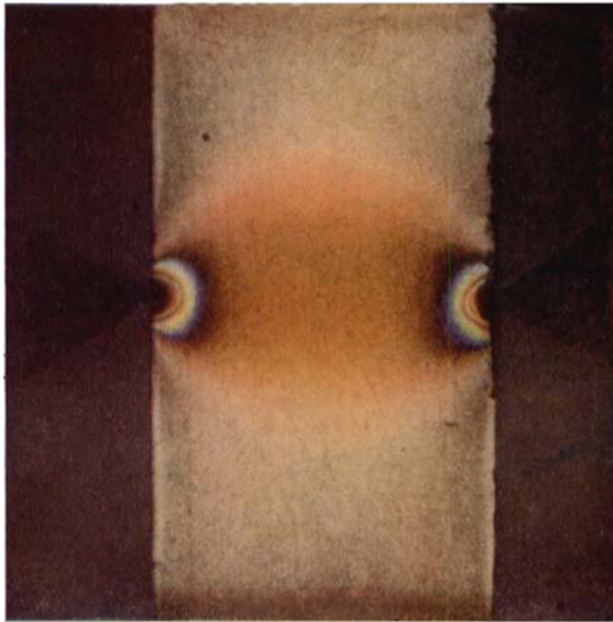
Fig. 29. The Stress in a Flat Tension Test Specimen of the Contour used by Prof. Dalby.
