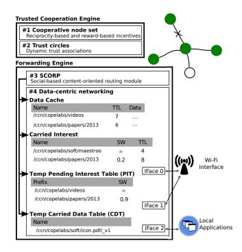
Figure 3. PDS node architecture for mobile citizen sensing.
