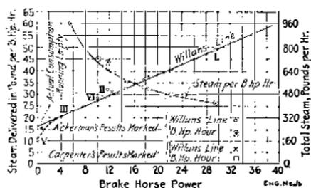
Fig. 8.—Diagram of Test Results on Low-pressure Engine.
