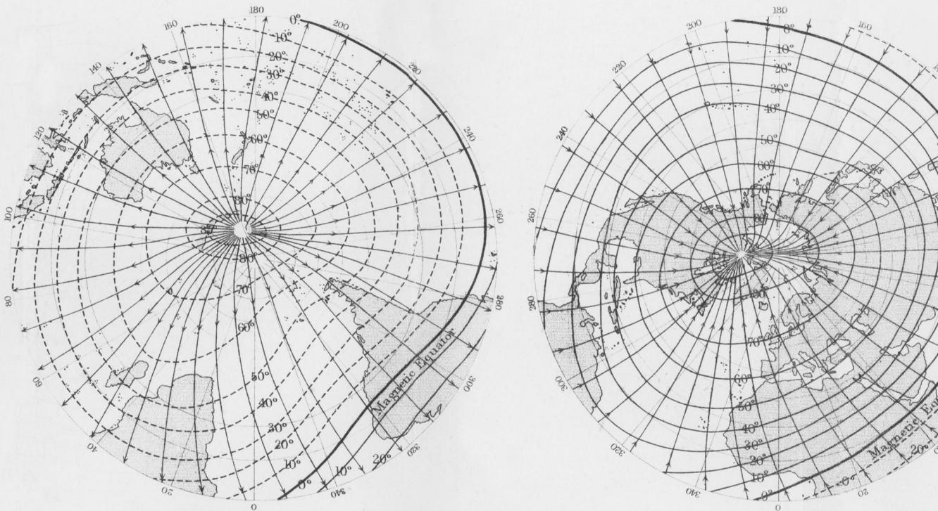
1. The Magnetic meridians, — or lines showing the angle made by the "line of force" with the Geographical meridians — are marked with arrow heads. The arrow heads also show the direction of the North end of the compass needle.
