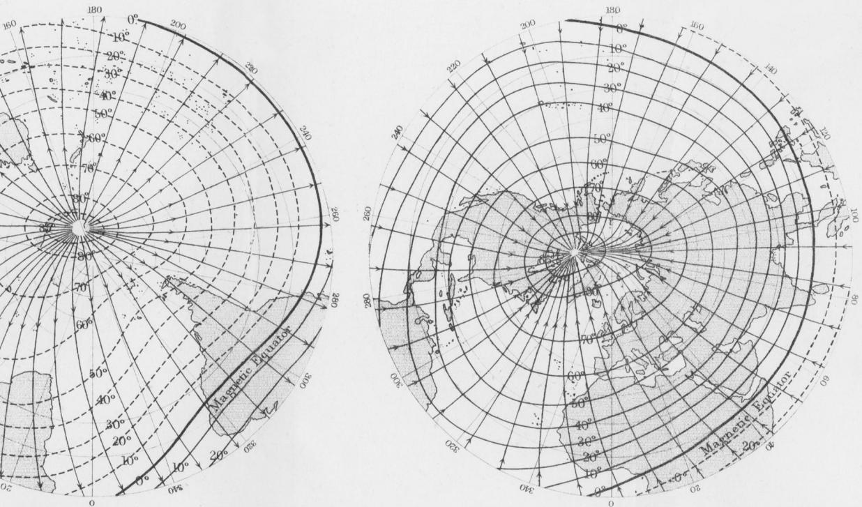
Magnetic meridians, — or lines showing the angle made by the "line of force" with the Geographical meridians — are marked with arrow heads. The arrow heads also show the direction of the North end of the compass needle. Lines passing through points of equal North Dip are shown by continuous lines: South dip by broken lines.
