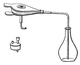
The bottle is then closed by a caoutchouc cap, having two tubular openings for the introduction of tubes. In the chemical laboratories of Germany, these caps are now almost exclusively used instead of perforated corks. One opening of the cap is closed with a round glass rod, and the other with a kind of funneltube, which enters the vessel to the depth of about two inches. This upper part of the funnel-tube is a wider tube, which can be closed with a cork.
