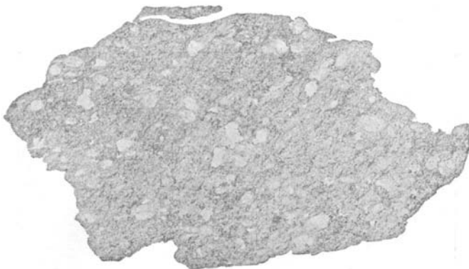
Fig. 2.—Natural size. Micaceous gneiss with sand-grains. Bed 130 (north) St. Gothard Tunnel.
