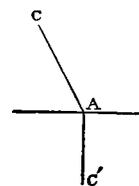
2d, That if the same heat  $Q$  originate in the medium, and strike  $A$  in the direction  $C'A$ , the quantity reflected back into the medium will be  $aQ$ , and the quantity refracted out in the direction  $AC$  will be  $(1-a)Q$ .
