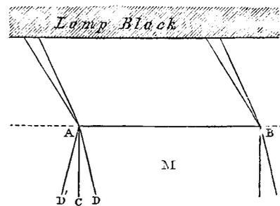
(M) may be maintained at this temperature, it is necessary that the heat which has left the surface AB, having come from the interior of (M), in the directions contained in any very small angle CAD, shall be replaced by an equal quantity of
