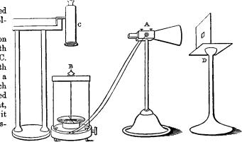
The heated body is placed behind the diaphragm, filling up the field of view from the cone; so that every ray reaching the cone from behind the diaphragm comes from the heated body.
