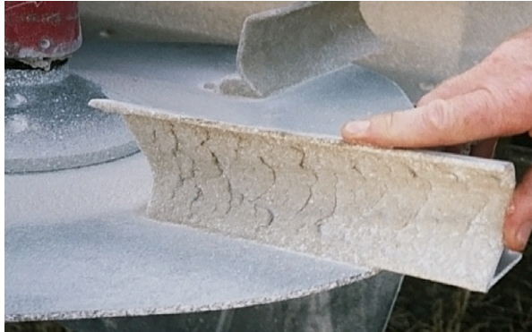
Figure 2. Build-up of fertiliser on vanes will affect the spreading pattern.
