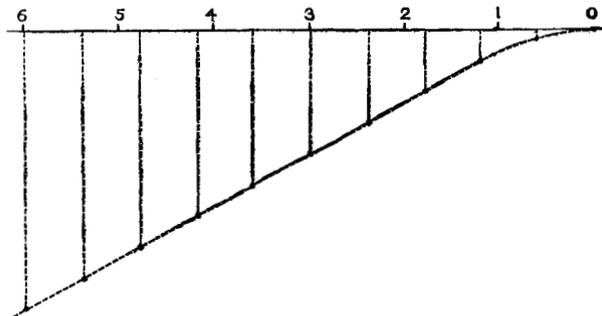
the form of the line drawn through such a series of balls, dropped from a vessel moving at the rate of 6 feet per second. The equations of motion are (Appendix, Problem I.)—
