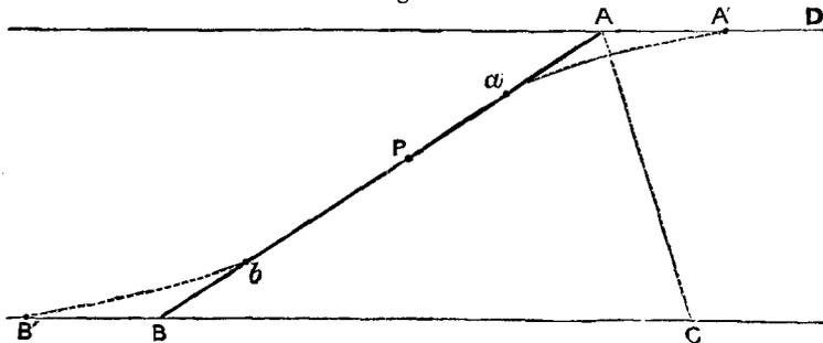
If the cable assumes the form of a straight line  $AB$  (Fig. 3), it is evident, that to bring it in order to lie straight at the bottom, the point  $A$  must move in the direction  $AC$ , bisecting the angle  $BAD$ , and that each point between  $A$  and  $B$  must move parallel to  $AC$ ; that is to say, the motion of every
