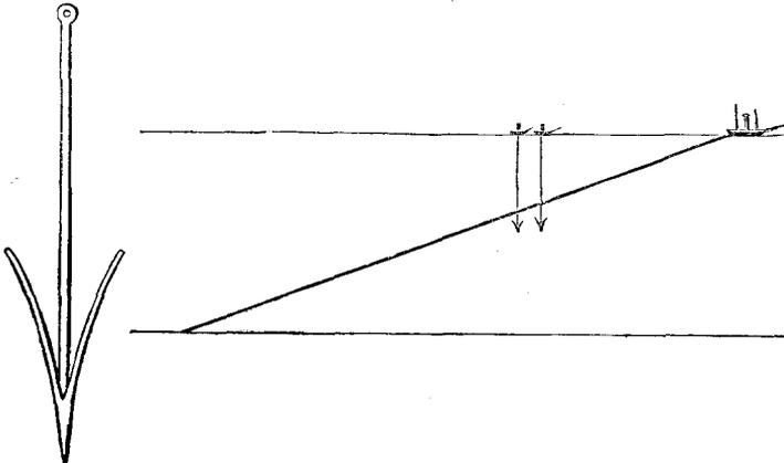
depth a little below the sinking cable. In case of fracture, upon a signal from the paying-out vessel, the two small vessels should at once steam at right angles to their former course, in opposite directions, so that one of them should cross the line of cable, which would probably be caught and jammed in the acute angle of the grapnel. As soon as this was done, which would be known
