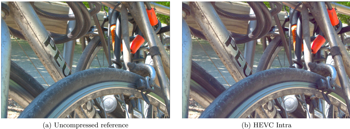
Figure 7: Central image ( u = v = 8 ) for content Bikes from LF data structure for reference and HEVC Intra for compression ratio R1.
