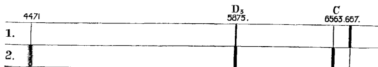
FIG. 1.—Diagram showing changes in intensities of lines brought about by varying the tension of the spark. (1) Without air-break. (2) With air-break.
