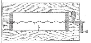
on it like a swivel, to keep the end of the helix true when the winch is turned. A little bead of wax is melted on each crest and hollow of the wave to represent particles, and the essential parts of the apparatus are complete. On placing it in front of the lantern, and focussing, a distinct and striking image of a moving wave with its vibrating particles is produced by turning the winch.
