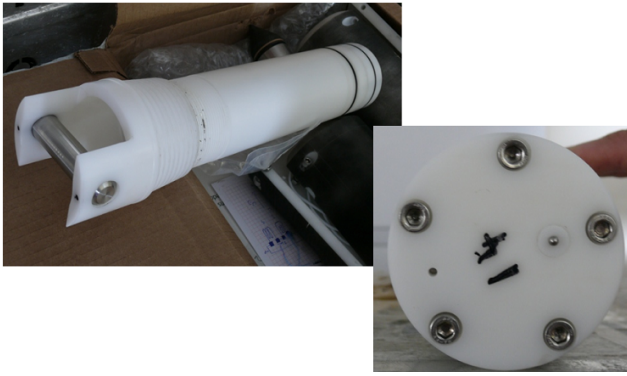
Figure 3. MeBoPLUG prior to being screwed into a MeBo drill pipe (left); photograph to the right shows bottom view into the borehole with ports for P (hole at left) and T (little pin at right) monitoring. See text.
