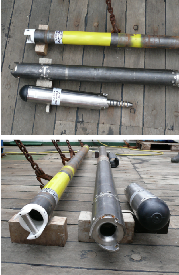
Figure 5. MeBoCORK A (i.e. autonomous) as well as MeBoPLUG for comparison. The MeBoPLUG is the white POM-made system screwed into the yellow rod, while the MeBoCORK-A is taken apart and has the actual monitoring and data unit with male hot-stab adapter taken out of its female counterpart. See text.
