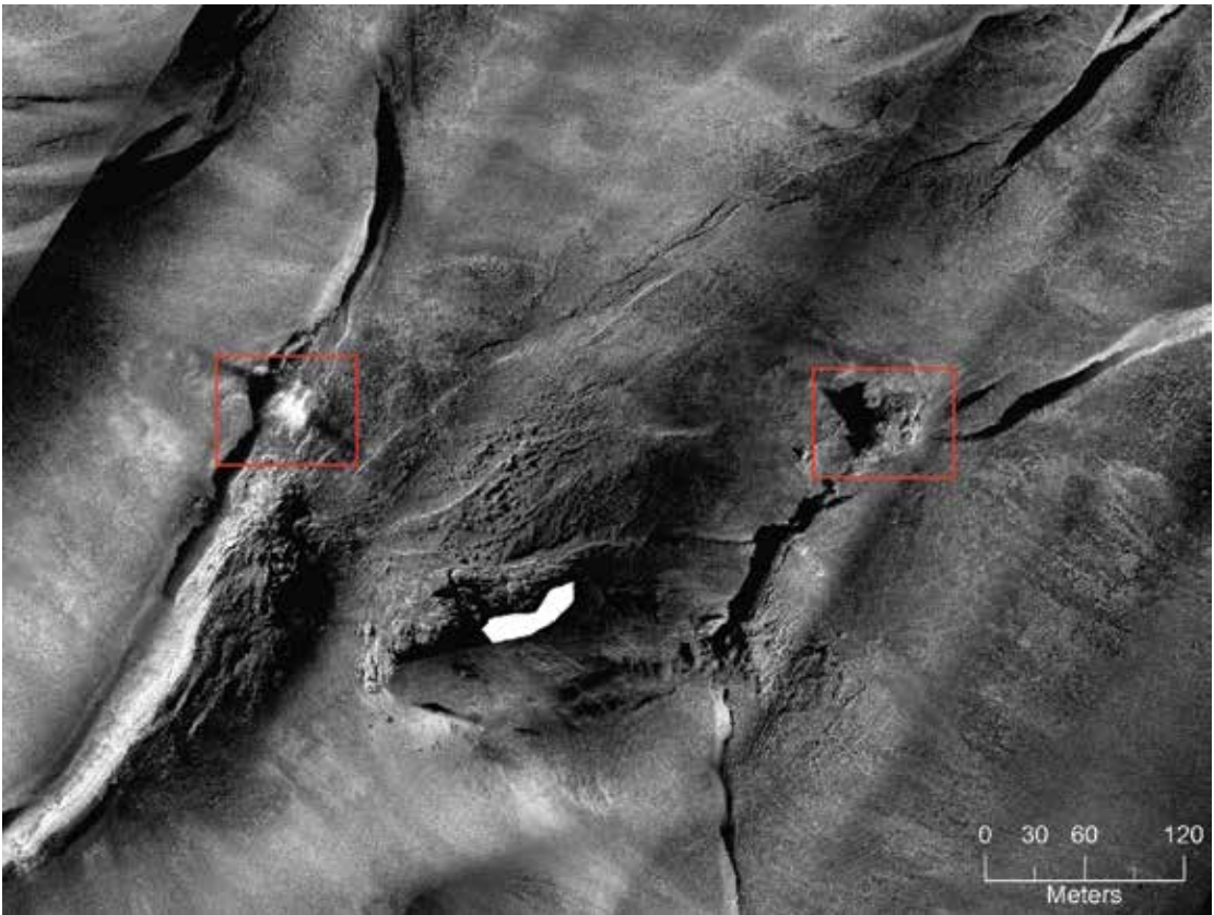
Figure 5: Overview of two new hydrothermal deposits discovered through multibeam sonar maps in 2013 and directly imaged during the summer of 2014. The vents, marked by red boxes, are visible by the mounds of hydrothermal debris and “flares” of hot water distorting the acoustic image.
