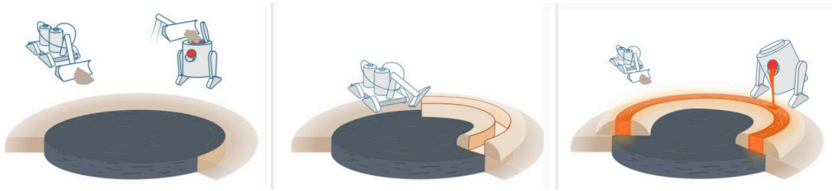
FIGURE 5. Illustration of the flow channel construction process, whereby the utility rover produces a controlled path within which the lava melt can flow and be constrained.
