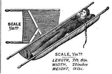
exceedingly simple—so much so as scarcely to need explanation, since the larger scaled section shows the method of opening and closing. The apparatus is inexpensive, and would be found serviceable in hospitals, police and fire brigade stations. The manufacturers are Messrs. Salt and Son, Corporation-street, Birmingham.
