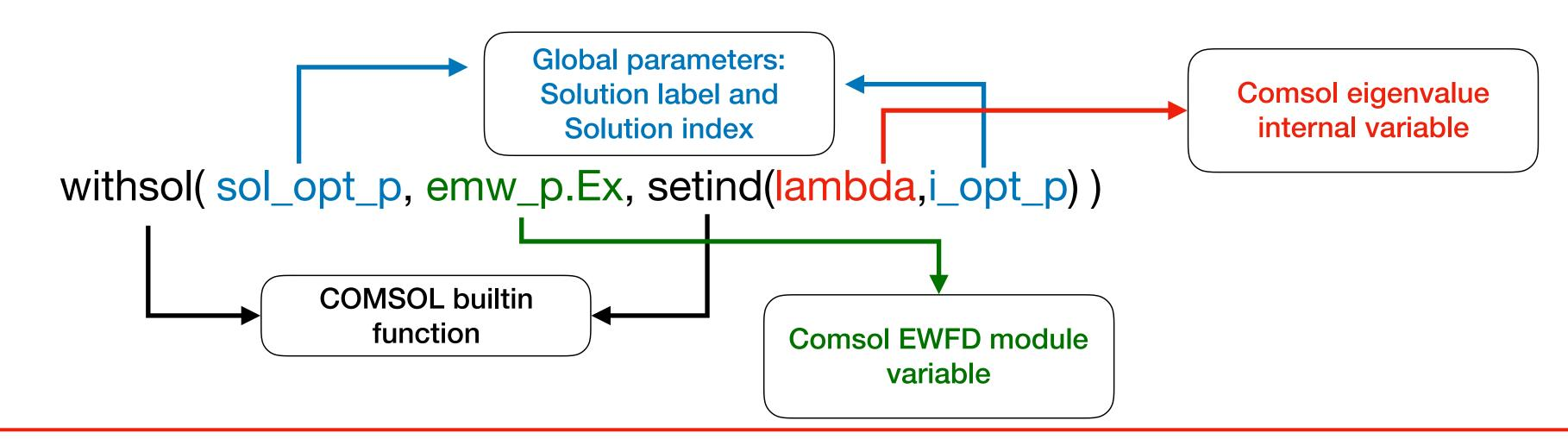
The output of the withsol() function is always the emw\_p.Ex field stored in 'i\_opt\_p' index of solution 'sol\_opt\_p'. This function will override, any selection of dataset during a plot or evaluation of this function.
