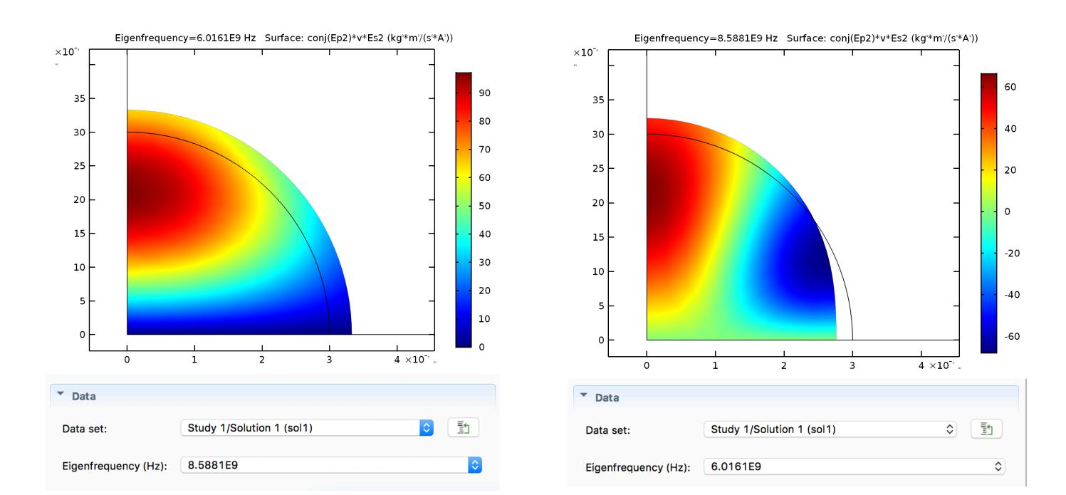
To be able to quickly skip through the several sought mechanical modes, the withsol() operator is **not used** in the mechanical solutions. This allows one to quickly choose the desired mechanical dataset (sol1) and the desired eigenfrequency to visualize the quantity of interest.
