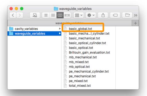
• • • basic\_global.txt ~ omega0 withsol(sol\_opt\_p,2\*pi\*emw\_p.freq.setind(lambda,i\_opt\_p)) "Pump frequency" beta\_p withsol(sol\_opt\_p,abs(emw\_p,beta),setind(lambda,i\_opt\_p)) "Pump mode wavenumber" beta\_s withsol(sol\_opt\_s,abs(emw\_s,beta),setind(lambda,i\_opt\_s)) "Stokes mode wavenumber" beta\_ac (beta\_p-signBS\*beta\_s) "Phase-matched Mechanical mode wavenumber"
