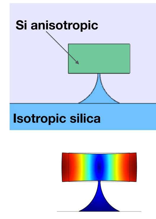
**Mechanical mode calculated** using anisotropic Si
