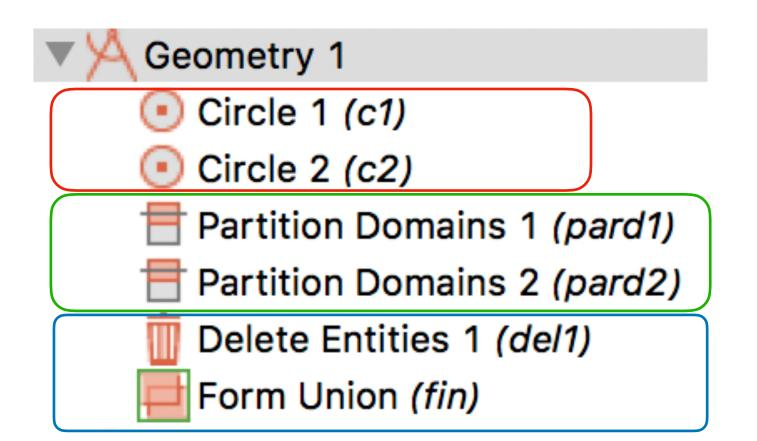
• If symmetries are not necessary, steps 2 and 3 above can be avoided. • Although it is not necessary to explore symmetries, it may lead not only to substantial computational time reduction but also easier selection of pump and scattered modes for intra-modal scattering.
