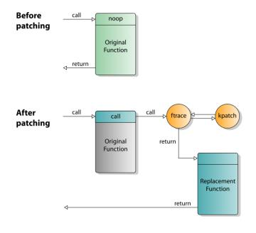
*Figure 3.* Live Kernel Patching by Kpatch Overview [7].
