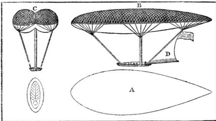
Let A B C represent the plan, side and end elevation of a balloon or aërial vessel, made of woollen cloth, and kept to its
