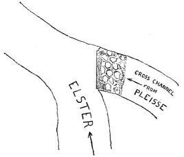
This beam was in constant vibration, being influenced by the currents of both streams, that of the Elster being the more active. Hence the ice was constantly subject to gentle shocks as it was pushed up stream by the beam, and as it came back again against it. The ice next to the beam, along the walls, which were of cut stone, and farthest from the beam, was of a slushy consistency, but the central portion appeared as roughly shaped hexagons.
