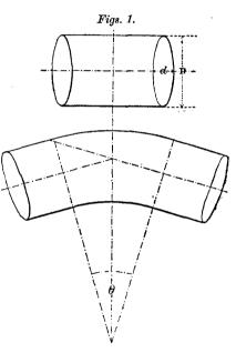
coincided perfectly with the surface of the pipe—showing that the anchor rods were doing the work for which they had been provided. To illustrate the magnitude of the forces to be resisted, it may be mentioned that in the cases of the 40-inch pipes used on the Thirlmere aqueduct, the unbalanced thrust at a bend of 34°, subjected to an internal pressure of 100 lbs. per square inch (and in some instances the pressures were as high as 180 lbs. per square inch), amounts to nearly 33 tons.
