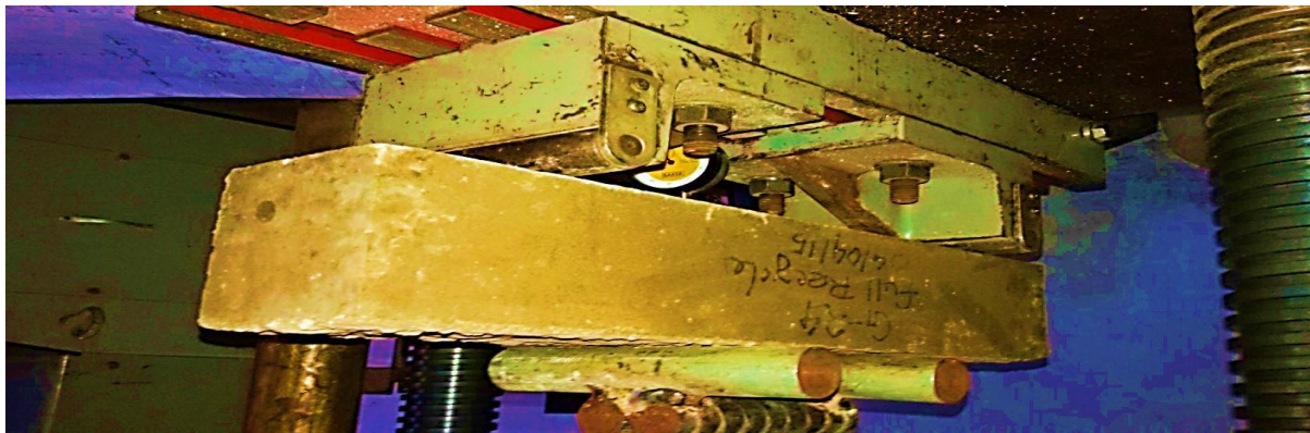
Fig: 4. Set-up of beam during flexural strength test
