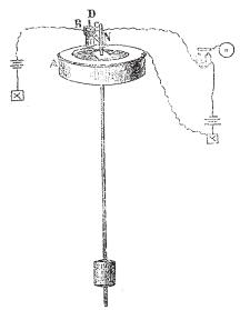
falls, breaks contact with B and makes contact with C, which thus tends to pull the needle over to C, and so on; in this way the pendulum receives at each oscillation the impulse necessary to overcome the forces tending to stop it; and thus will keep oscillating as long as the battery supplies the motive power. For small arcs the beat is not affected by variation in battery
