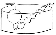
as large a surface as possible to the ethylene, in order that combination may be effected. An ordinary bulb wash-tube (fig. 2) answers for this purpose. Into such a tube, chloride of sulphur was brought, and dry ethylene allowed to bub-
