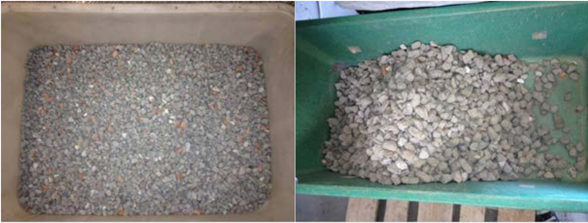
Figure 6: Grey concrete fractions obtained from MRA after UV-VIS sensor-based sorting (left: 6-12 mm, right: 20-35 mm).
