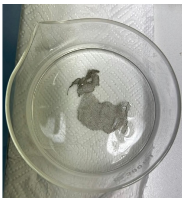
Figure 1. a) dissolving tungsten powder in hydrogen peroxide and b) the reaction of the remaining hydrogen peroxide at Pt mesh
