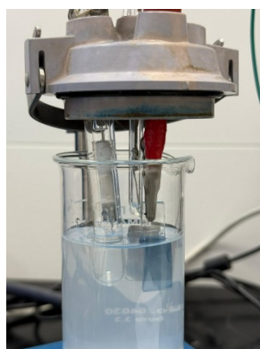
Figure 2. Three-electrode system for electrodeposition of \text{WO}_3 and modified \text{WO}_3
