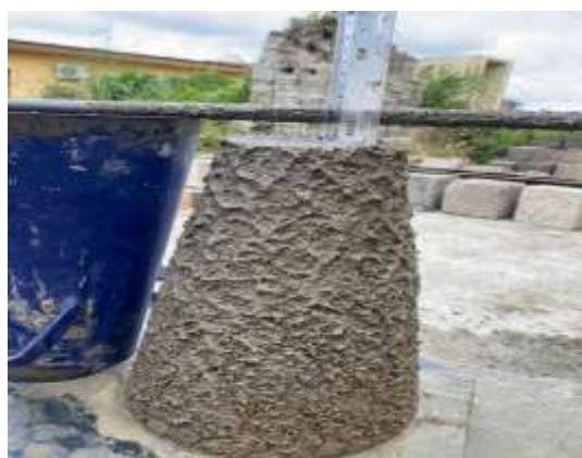
Plate 2: Slump test of the fresh concrete
