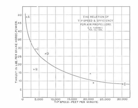
The curve shown herewith gives the whole thing in a nutshell. For any propeller, of rational design, the higher the speed the lower the efficiency, and for any type, the larger the diameter the greater the efficiency.
