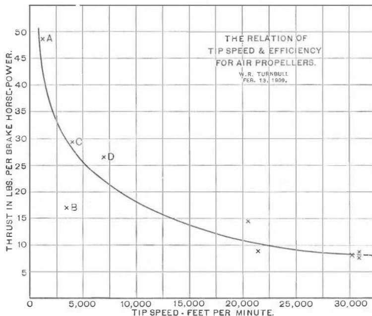
The curve shown herewith gives the whole thing in a nutshell. For any propeller, of rational design, the higher the speed the lower the efficiency, and for any type, the larger the diameter the greater the efficiency.
