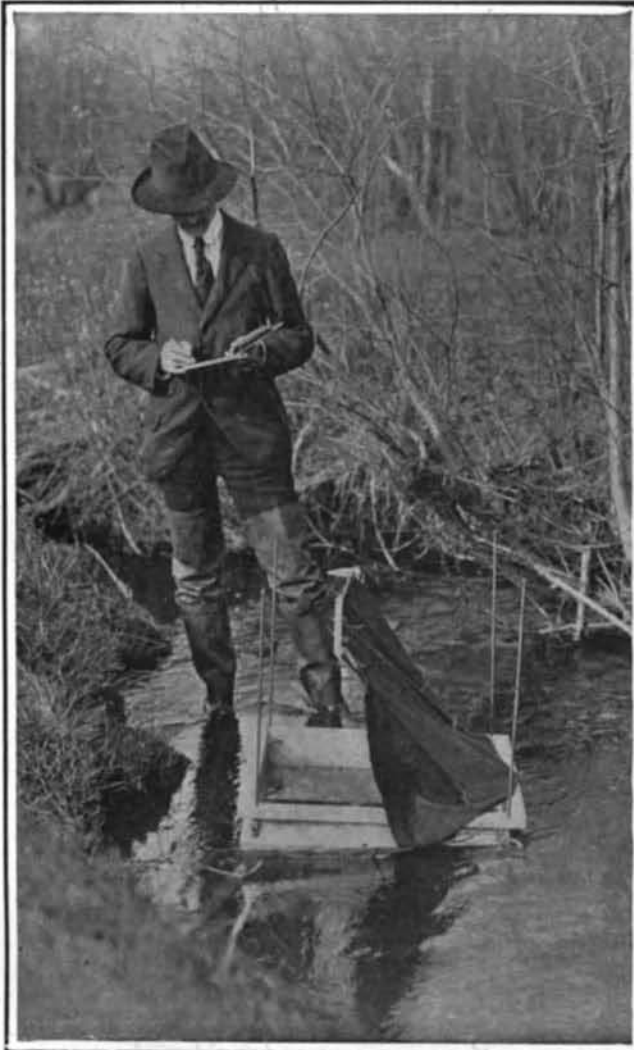
Fig. 3.—Two-foot water glass for studying lampreys.
