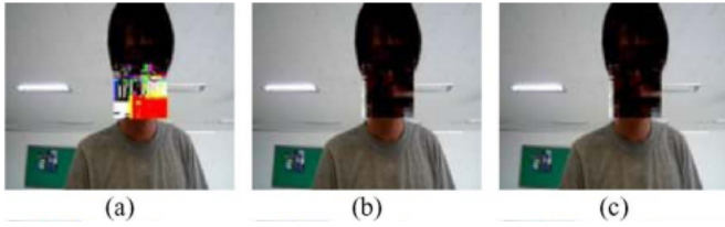
Figure 2. Visual effect of ROI-based, subband-adaptive scrambling[13]. (a) all subbands. (b) DC+LP+HP. (c) DC+LP.
