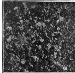
FIG. 2.—Alloy containing copper 80 per cent., zinc 20 per cent., annealed at 700^{\circ} .
