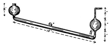
When the combustion is complete and pure air or oxygen has been passed long enough to expel all carbon dioxide, the absorption apparatus is disconnected and the contents filtered.
