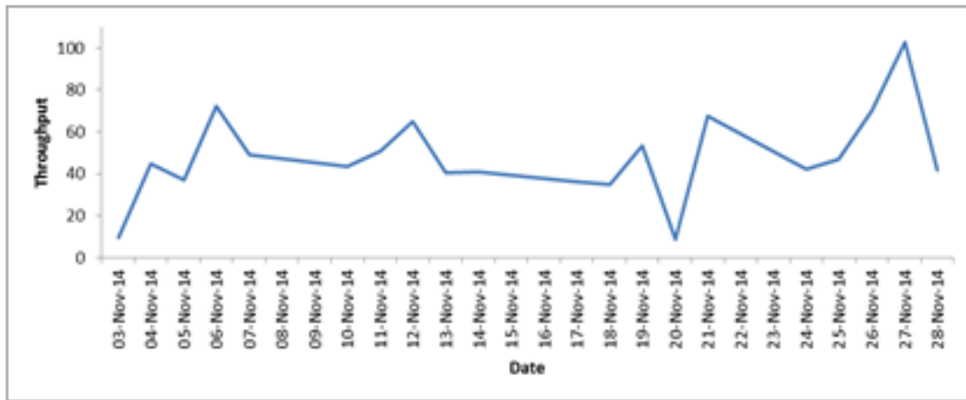
Figure 43: Daily throughput prediction using the Weibull distribution from one sample iteration
