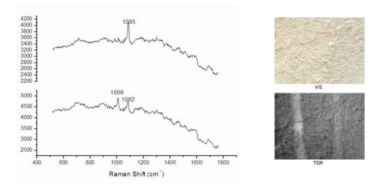
Fig. 1: Analysis of plaster decay in fresco test-beds (example). Left: Raman spectrum of sound (top) area and sulphate decay (botton); Right: VIS image and TQR response (sulphated areas are the vertical lines).
