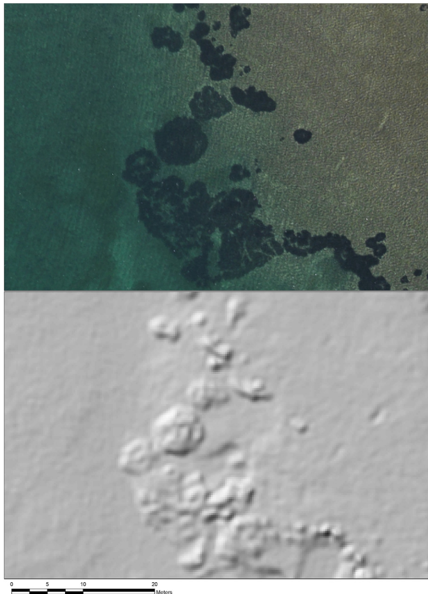
Fig. 16. Sv. Petar. Upper image: orthophotograph of an area partly covered with seagrass (dark green). Lower image: shaded DTM of the same area after filtering. The dense seagrass was not removed by the filter algorithm. North is up. (For interpretation of the references to colour in this figure legend, the reader is referred to the web version of this article.)
