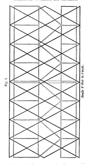
The Author of the Paper proposed a lantern with a new arrangement of framing, as shown in Plate 4, Fig. 43, having partly vertical and partly inclined framing; all of which was to coincide optically with the armature of the dioptric apparatus. Now, with the heavy vertical armature of the early dioptric apparatus, where on the bearing of each vertical portion of the arma-
