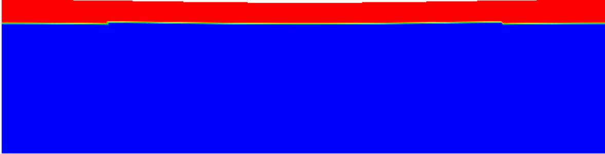
Figure 63: Setup for the topography relaxation benchmark. The box is 2800 km wide and 700 km high, with a 100 km lid on top. The lid has a viscosity of 10^{23} Pa s, while the mantle has a viscosity of 10^{21} Pa s. The sides are free slip, the bottom is no slip, and the top is a free surface. Both the lid and the mantle have a density of 3300 \text{ kg/m}^3 , and gravity is 10 \text{ m/s}^2 . There is a 7 km sinusoidal initial topography on the free surface.
