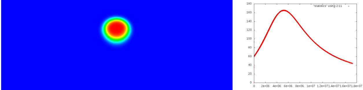
Figure 23: Evolution of surface topography due to a rising blob. On the left is a snapshot of the model setup. The right shows the value of the highest topography in the domain over 18 Myr of model time. The topography peaks at 165 meters after 5.2 Myr. This cookbook may be run with the cookbooks/free-surface.prm input file.
